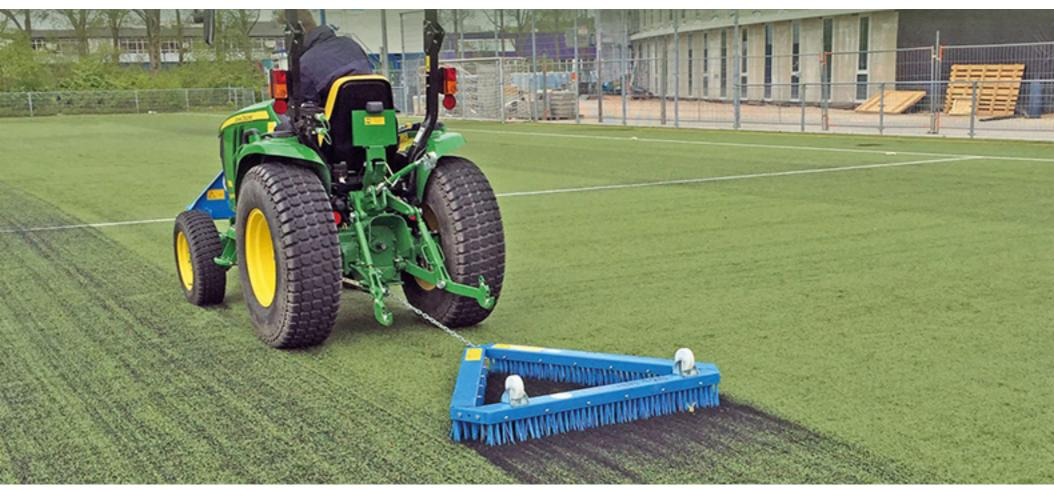
The Tbrush is a triangle brush that can be used for the daily maintenance of your synthetic turf pitches. This, our most straightforward brush, has been constructed with a premium steel frame in combination with completely synthetic brushes. These synthetic brushes provide you with a major advantage, since they will not decay due to the effects of water.
