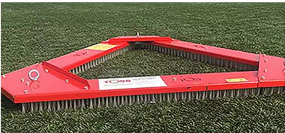
The Tbrush is suitable to brush synthetic turf pitches with several types of infill; for instance, rubber, zand, or cork. When you brush your pitch on a regular basis, it can prevent reduced drainage, deteriorated sport technical
